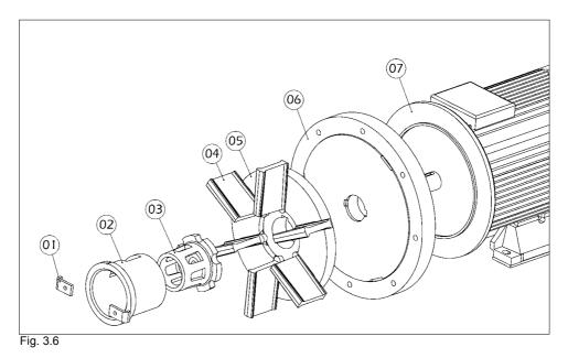
Around the centre of the blast wheel there is the impeller feeding dosed quantities of abrasive onto the blades of the turning blast wheel. On top of this is the control cage (with 2 notches) which, once it is carefully set, regulates the flow of abrasive.
